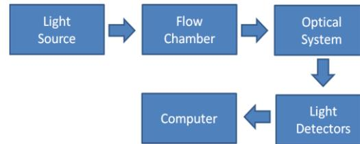
The flow rate of sheath fluid will determine how rapidly the stream of material will move, and thus reach the laser(s) of the cytometer. In an ideal situation, material will pass through the laser one-by-one, and thus data from each individual cell ('event') will be recorded. This will provide the most accurate results and it is therefore very important to understand the capabilities of your cytometer.
