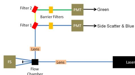
A bar placed on the opposite side of the flow chamber blocks the laser beam. The forward light scatter (FSc) detector sits behind the blocker bar and this detects light scatter at angles in a forward direction. Forward light scatter is an indication of cell size.
